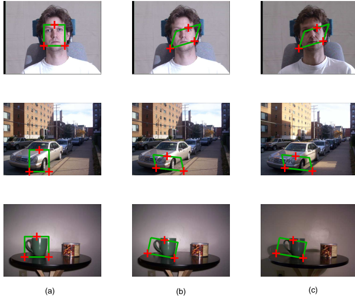
Figure 1. (a) A template centered around the object of interest with three canonical points shown as red pluses. (b) Sample warps defined by the random perturbation of the three canonical points. (c) Sample warps shown on an image that has different illumination conditions as compared to that of the template for various objects.
